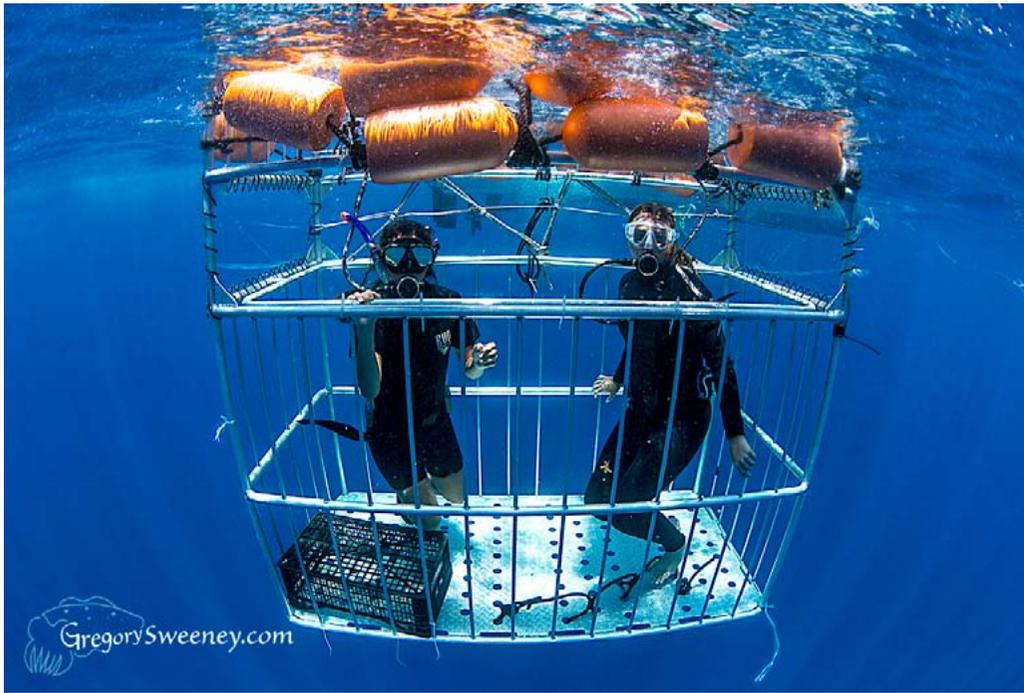
*The cage fits 2 people with a hooka air supply located in the boat. It has Lexan polycarbonate panels on the sides and one large one in the front with 2 open ports facing front.*
